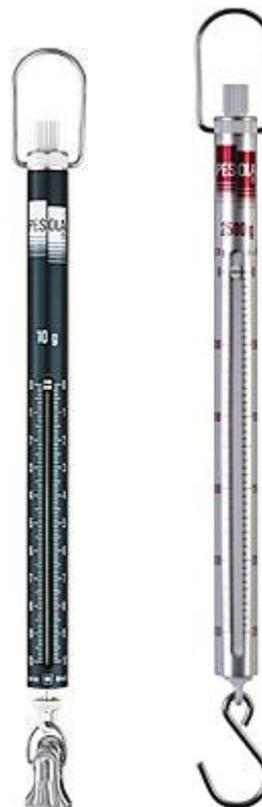
Federwaage (Made in Switzerland)
