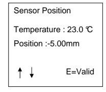
This indicate the force sensor position in front of surface of sample:
