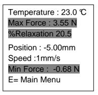
The Max Force is the maximum force measured during the compression time.
