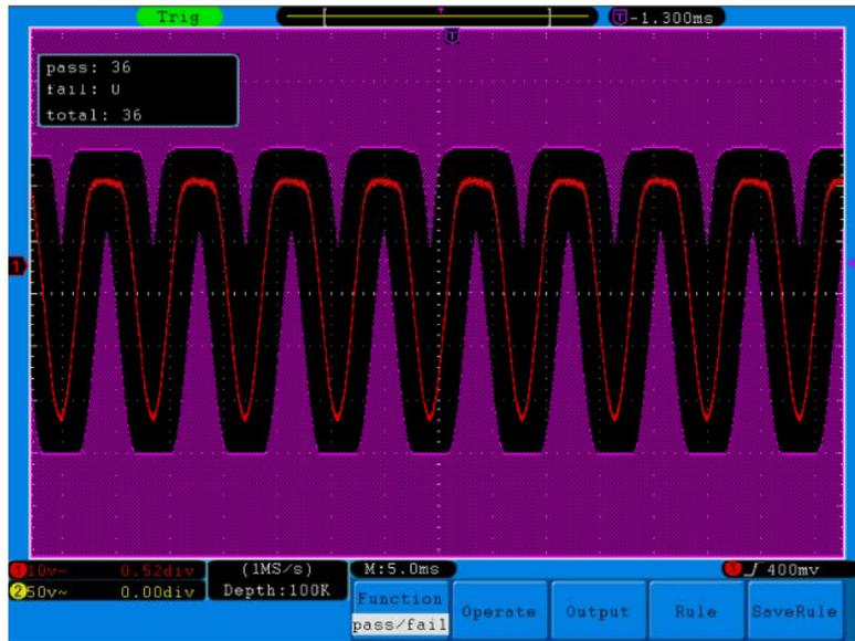
Fig. 58 Pass/Fail test
