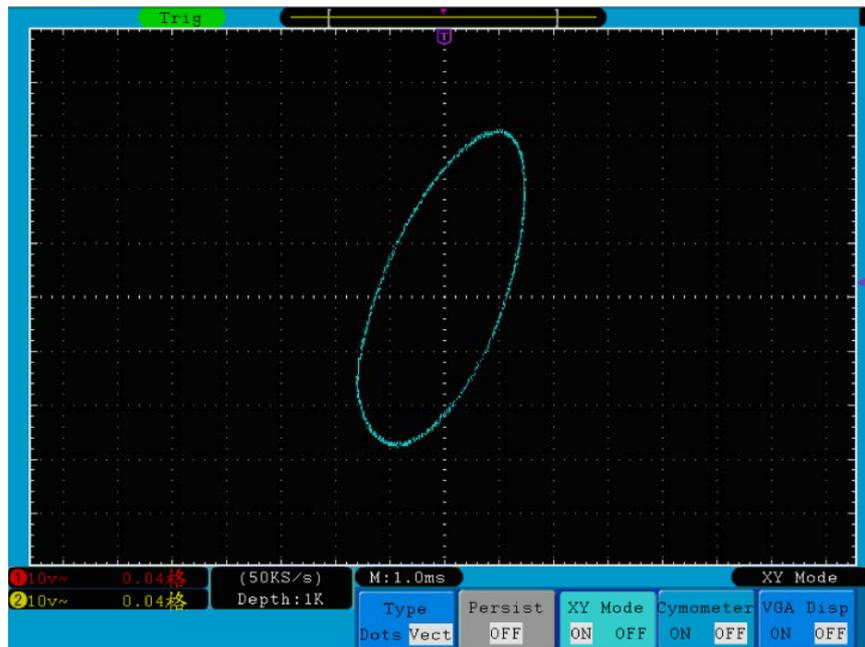
**Fig. 46** XY Display Mode
