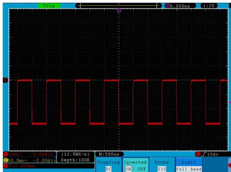
Fig. 18 Waveform Inverted
