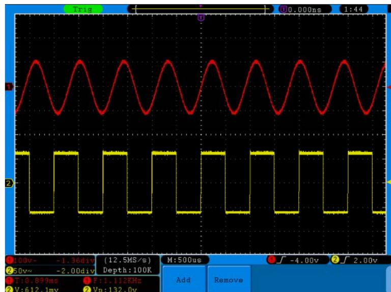
**Abb. 68** automatic measurement
