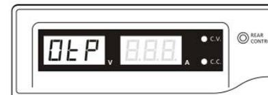
Check your load and output setting. Allow the unit to cool down for at least 30 minutes.
