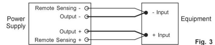
**The remote sensing wire should be AT LEAST 22AWG wire size.**
