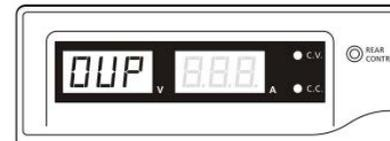
To reset the warning, switch off the unit and remove all loading.
