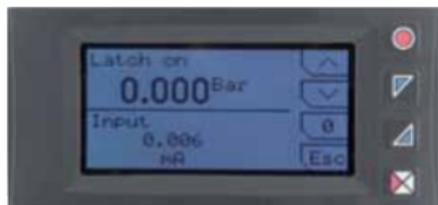
To use the LATCH ON function: enter configuration, select **Setting** on par. 8 **Latch on** and press **Sel** (UA964801 shows the page in the picture).
