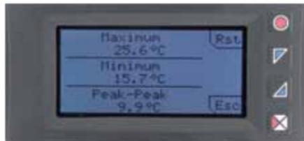
The UA964801 is provided with a page for the visualization of peak values: max. peak, min. peak and peak-to-peak of analogue input. Keeping pressed **Rst** it is possible to reset the visualized values.
