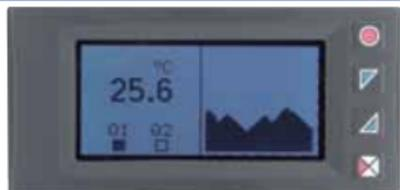
This page displays the process, the relays status and a graph representing the process trend.
