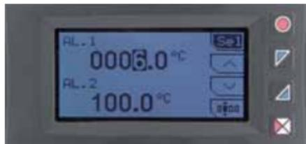
Press **Setpoint** to enter the thresholds modification.
