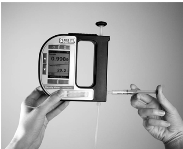
Fig. 10 - 2 Filling sample using the plastic syringe
