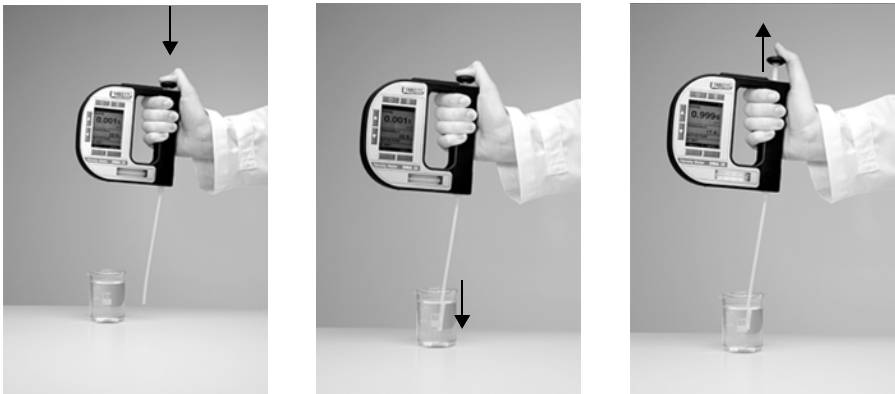
Fig. 10 - 1 Filling sample using the filling tube
