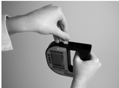
Fig. 12 - 4 Opening the battery cover
