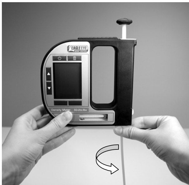
Fig. 7 - 1 Connecting the filling tube
