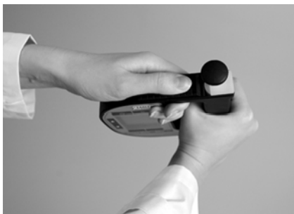
Fig. 12 - 1 Removing the pump
