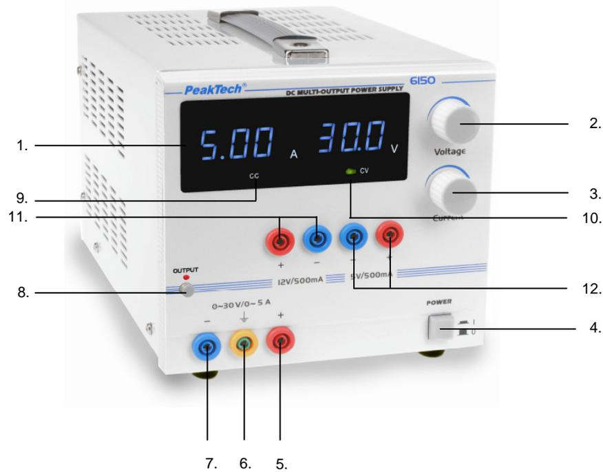
1. Amp and Volt display: indicating output current and voltage
