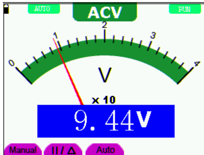
figure 23: AC Voltage Measurement
