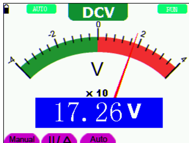
figure 22: DC Voltage Measurement
