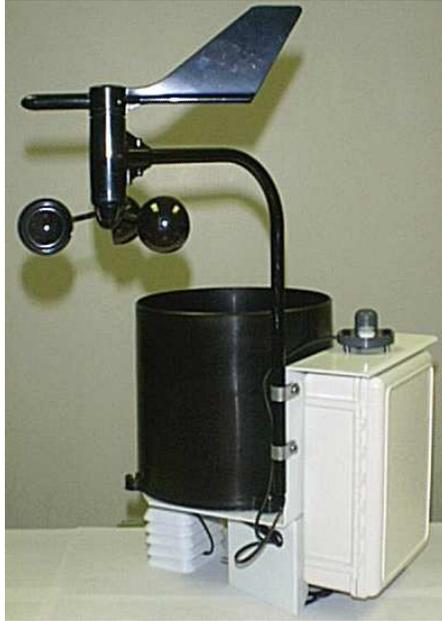
Apart from the anemometer, the WatchDog Weather Station comes fully assembled and ready to mount. The anemometer arm is attached to the enclosure back plate with two clamps. After positioning the arm, the screws should be tightened to secure it in place.
