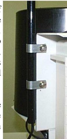
*Anemometer clamped to back plate (for visibility, black, rubber clamps not shown)*
