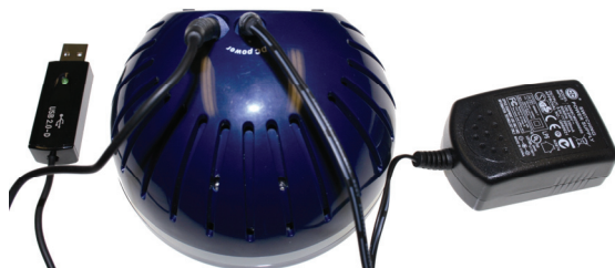
Fig. 5: Rear side of the Wöhler CDL 210 with USB cable and power supply
