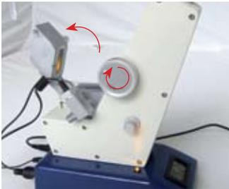
Turn the locking knob to lift up the illumination prism.
